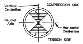
The above is a graphic representation of the degrees of stress in the wall of the tube when the beam is under load. The length of the arrows "X" represents the amount of stress at a given point. From this illustration, it is evident that the two opposite stresses diminish as the horizontal center line of the beam is approached.
