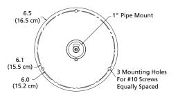
Built-in permanent/1-inch pipe mount polycarbonate base.
