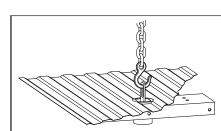
distorted downward from heavy use. If you use an overhead-lifting device, it should be disconnected before squaring the center section across the frame, installing the sideplates and torquing fasteners.
