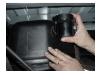
Step 3: Slide fuel valve from bracket.
