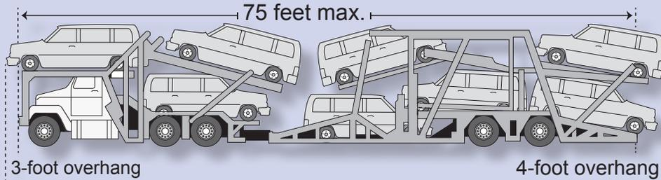
To qualify as an automobile and boat transporter, the stinger-steered vehicle may carry cargo on the power unit behind the cab and on an over-cab rack.
