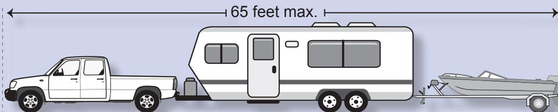
Combinations of three vehicles, whether truck-trailer-boat, or motor home-boat-car, are limited to 65 feet overall length.
