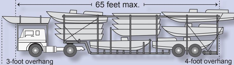
To qualify as an automobile and boat transporter, the conventional transporter may carry cargo on the power unit behind the cab and on an over-cab rack.
